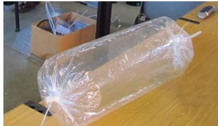
*Figure 5: Air sample bag to be send to the laboratory for olfactometric analysis*
