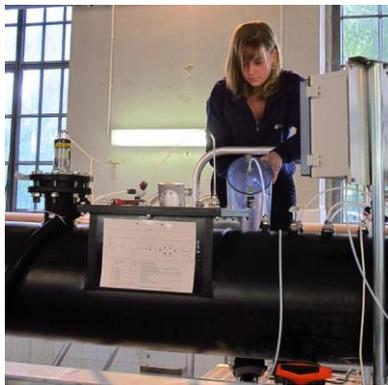
*Figure 4: Sampling from the headspace of the sewer research plant*
