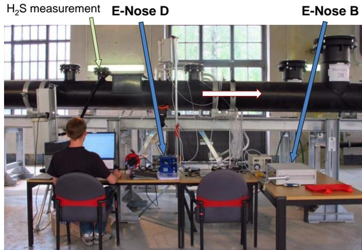
Figure 2: Measuring site of the e-noses at the sewer research plant; flow direction of the wastewater is indicated.
