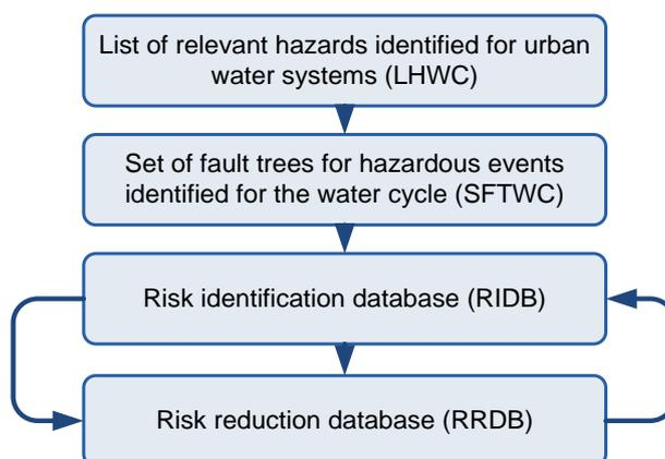
Figure 2 – Tools developed to support application of the WCSP framework
