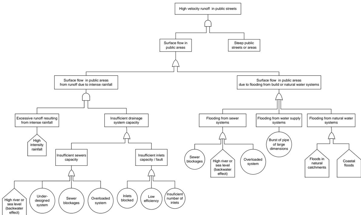
Figure 3 – Example of a fault tree for the hazard ‘High velocity runoff in public streets’
