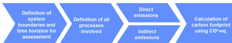
Figure 6 – Process to calculate the carbon footprint of a risk reduction measure
